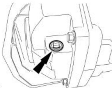
3. Clean the drain plug. Apply threadlock and sealer to the plug threads and install the drain plug.
