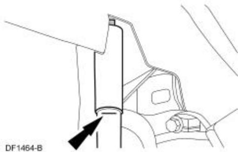
5. Remove the clip and disconnect the parking brake cable from the rear caliper.
