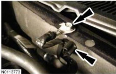
10. Install the 2 cowl vent screen plastic rivets.
