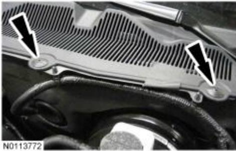
10. Lift the cowl screen and remove the ground strap bolt.
