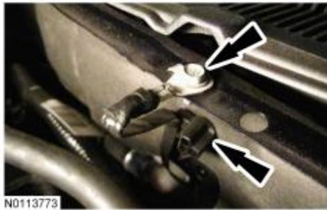
11. Disconnect the brake booster vacuum hose quick connect at the engine.
