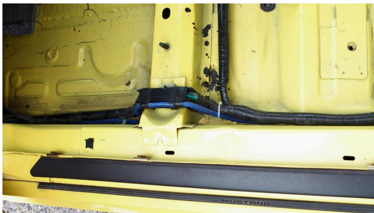
Figure 3 - Amp Power Cable by Driver Seat
