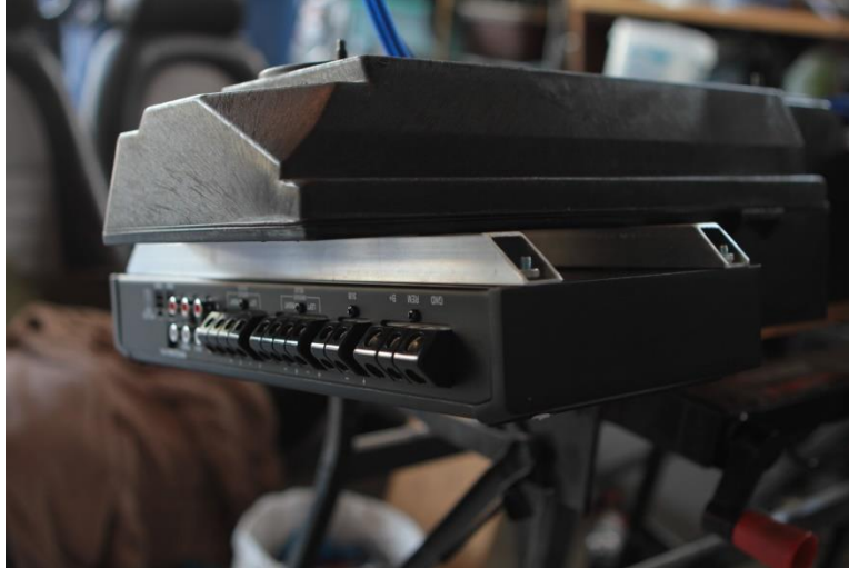
Figure 12 - Mounted R600X5 Amplifier
