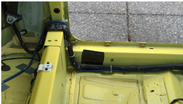
Figure 4 - Cable Routing Over Rear Seat Hump
