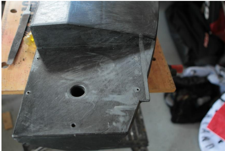
Figure 11 - Sound-box Modification for Amp Mounting
