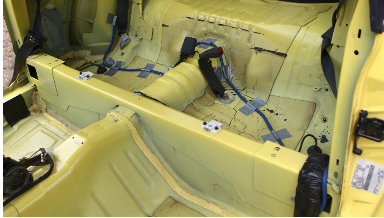
Figure 5 - Under Rear Seat Routing
