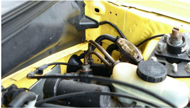
Figure 2 - Cable Running Through Firewall
