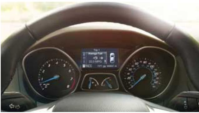
speedometer, fuel gauge, and engine coolant temperature gauge, as well as an Intelligent AWD gauge and the currently selected gear (in SelectShift mode), if equipped. Exact features may vary based on your vehicle's configuration.
