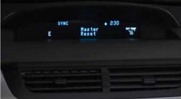
Press the **Arrows** or **Seek** buttons until **Master Reset** displays on the screen. Press **OK**.
