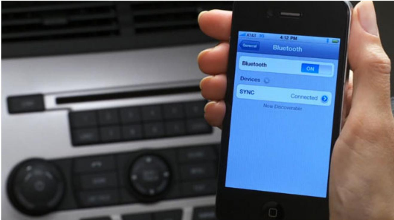
To use any of the phone features for SYNC<sup>®</sup>—such as making a call or receiving a text message—you must first connect, or "pair" your Bluetooth<sup>®</sup>-enabled phone. Pairing is what allows Bluetooth devices to communicate securely with each other.
